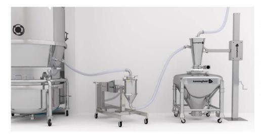
In the left example, material is drawn by vacuum from a fluid bed dryer bowl through a Uni-Mill and collected in a Uni-Filter. A suction blower package not shown provides the motive force for material conveying.
