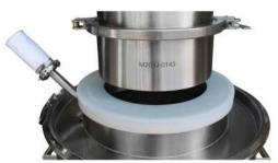
Left: a silicone cap and penetration create an interference seal when the milling head is lowered. This is mostly used for non-hazardous dusts where the intended purpose is for general dust containment. A second drum lifting inverting post can be used for contained feeding.
