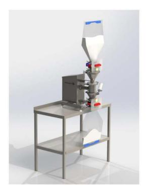
In all solid "container to container" milling applications, the displacement of air from the discharge container as it fills may require venting. This happens when the air or gas in the lower container cannot percolate upward through the mill and through the bed of powder contained in the upper feed container. When using plastic charge and collection bags, the bags can be manipulated to force air or gas from the collection to the feed bag. This avoids the use of vents and vent filters.
