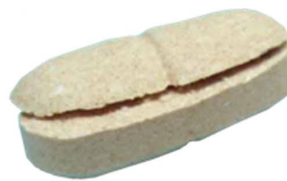
Photo example of capping
