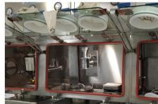
In the case of the oscillator this would be extremely challenging to design and manufacture. On the other hand, the underdriven Uni-Mill is a natural fit requiring only minor modification to allow isolator integration with total separation of process and utility/drive components.
