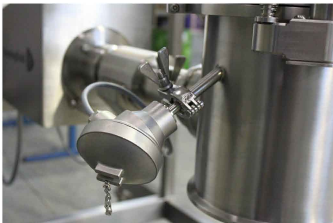
Figure 2: Temperature probe located against screen of a conical mill
