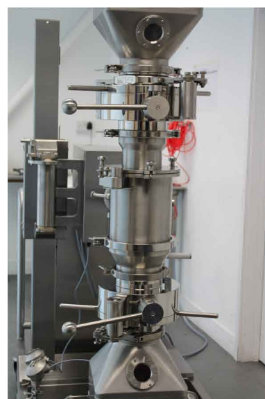
Figure 1: Conical mill with high containment split valves installed on inlet / outlet
