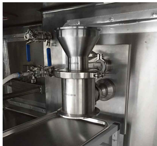
Figure 2: Isolator milling - the milling head is contained within the isolator, with the motor and controls mounted externally
