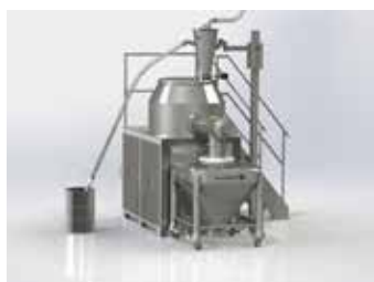
Vacuum Transfer into a High Shear Mixer
