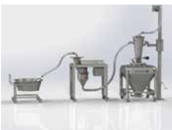
In-Line Vacuum Transfer Milling
