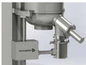
Wet Milling (Post-Granulation)
