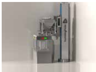
Lifting IBC above Tablet Press
