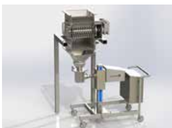
Pre-Break Before Milling
